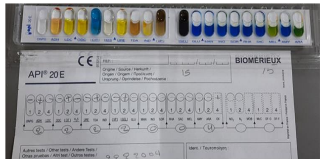
Fig. 2 Biochemical assays for Gr- bacteria and positive for the oxidase test of pseudomonas aerugenosa using the API system
